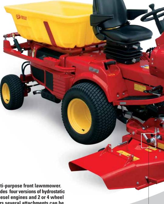
**SR machines** are multi-purpose front lawnmower. The SR product family includes four versions of hydrostatic machines with petrol or diesel engines and 2 or 4 wheel drive. With SR lawnmowers several attachments can be fitted to ensure an increased return on investment for landscapers and other professionals.
